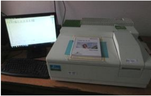
Fig. 5. Perkin-Elmer Lambda 25 UV-VIS Spectrometer Fig. 6. Absorption spectra of a liquid sample
