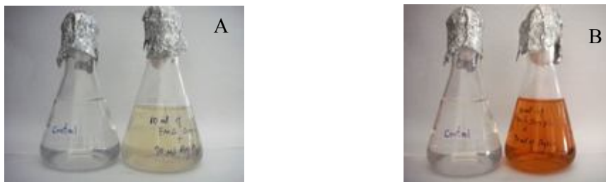
Fig 3. Synthesis of silver nanoparticles from the extract of Calocybe indica A=Before synthesis of AgNPs B= After synthesis of AgNPs.
