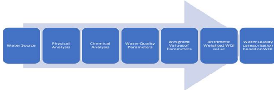
Fig. 2. Protocol followed for determination of the water quality index.
