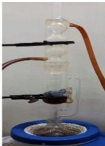
Figure 1. Soxhlet apparatus used for extraction of Solanum xanthocarpum leaves
