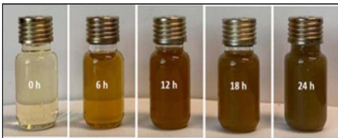
Figure 2. Visible observation of silver nanoparticles with different Time The particles were validated for the presence of a maximum absorbance peak at 400 nm in the UV-Vis spectroscopy. Optimized reaction parameters for synthesis of stable AgNPs were addition of 5 mL of AI-extract to 45 mL of \text{AgNO}_3 (1 mM) at pH 7 and incubation at 25\pm 1^\circ\text{C} in dark at 200 rpm. AgNPs were stable in all the five solutions tested shown in Figure 3 & 4.
